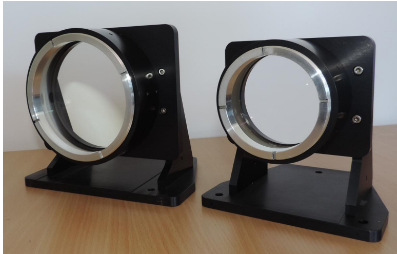
Fig. 8: BATMAN fore-optics lenses (doublet and triplet), mounted and aligned in their barrels.
